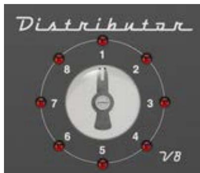
The rotor lamps show the state of the voices, on or off, and the rotor arm points to the next voice that will be allocated. As soon as a voice is used, Distributor's rotor arm moves to the next available position according to the Order and Pattern settings. Only voices that are off will be chosen unless Freeze is held or all voices are full.
