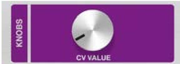
The Knobs section is where you'll find The Knob referred to by the name kn0b. The knob controls the level output from the CV output jack. The knob can turn from -120° counterclockwise to 120° clockwise with 0° being straight up.
