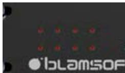
The LEDs show when an audio output has an active signal. There is an LED for each audio output.
