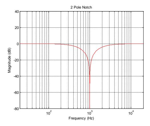
The two pole notch filter offers infinite attenuation at the cutoff frequency.
