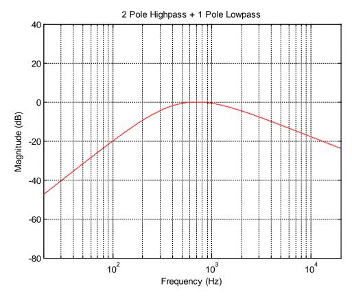
This is a two pole highpass and one pole lowpass combined filter. The rolloff is 12 dB per octave for the highpass section and 6 dB per octave for the lowpass section.
