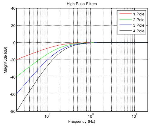
1 Pole High: A one pole highpass filter offering -3 dB at the cutoff frequency and 6 dB per octave rolloff.
