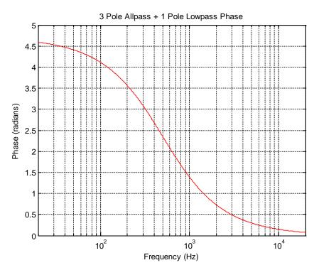
This is a three pole allpass and one pole lowpass combined filter with 6 dB per octave rolloff.
