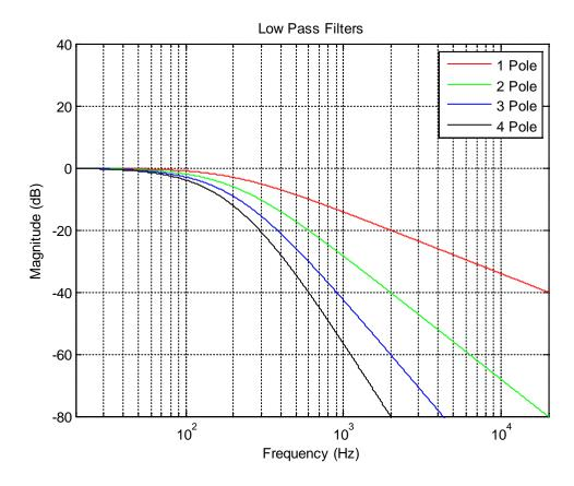
1 Pole Low: A one pole lowpass filter offering -3 dB at the cutoff frequency and 6 dB per octave rolloff.
