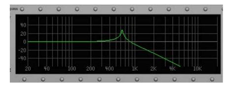
The display screen shows the filter frequency response. The x axis is logarithmic frequency. The y axis is magnitude in decibels.
