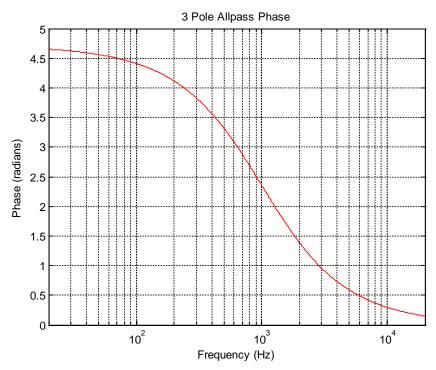
This is a three pole allpass filter. The plots show the filter with cutoff set at 1 kHz.
