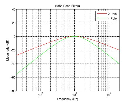
2 Pole Band: A two pole bandpass filter offering -0 dB at the cutoff frequency and 6 dB per octave rolloff in both directions.
