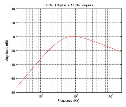
This is a three pole highpass and one pole lowpass combined filter. The rolloff is 18 dB per octave for the highpass section and 6 dB per octave for the lowpass section.
