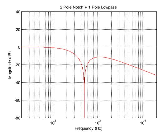
This is a two pole notch and one pole lowpass combined filter. The rolloff is 6 dB per octave for the lowpass section and infinite attenuation at the cutoff frequency, shown at 500 Hz.
