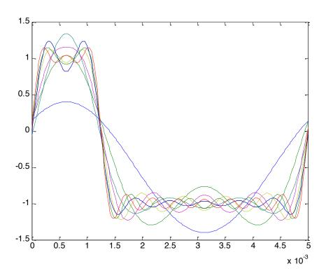
Now that you are thinking about sums of sine waves, the Ratio knob will make more sense. The harmonic amplitudes stay the same, but instead of each harmonic being at the harmonic number times the fundamental, they will be spaced by the ratio times the fundamental. So for an A4 note with a ratio of 3 the following frequencies result.
