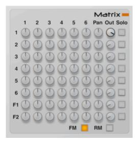
The matrix is where the FM/RM action takes place, as well as panning, output volumes, solo, and routing to the filters.
