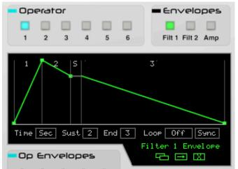
For example, the filter 1 frequency envelope is being shown on the display.
