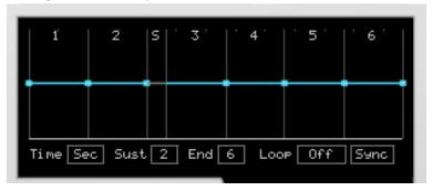
Each envelope can have up to six stages. The number of stages is set by clicking the "End" number. The level and time of each stage can be adjusted by clicking and dragging the points at the end of each stage. By clicking and dragging in the middle of each stage you can adjust the curve. You can use Reason's standard modifier keys for fine control or resetting of envelope parameters. (ctrl on Windows or command on Mac for reset, shift for fine control)
