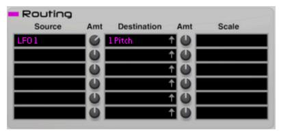
In this example, LFO 1 is modulating the pitch of operator 1. Modifier X is used as a scale so that it controls the amount of modulation that occurs. The small arrows in the Destination displays provide a drag-to-connect feature. Click on the arrow and drag to the desired destination knob to automatically select the destination. Reset the destination to Off clicking while holding the standard Reason modifier key (ctrl on Windows or command on Mac).
