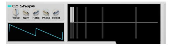
The lower area of the Harmonics Editor adjusts the phase of that particular harmonic. In the following plot, harmonic 2, the green sawtooth, has had its phase changed to 58 degrees. It has in effect been shifted to the left compared to the blue one, so the first peak is now outside the plot area. When the two sawtooths are summed they create a different final waveform.
