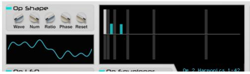
The Harmonics Editor lets you duplicate the operator waveform shape at multiples of the fundamental frequency. The duplicated waveforms are summed to create the final waveform. For example, if you play an A4 on the keyboard, the fundamental frequency is 440 Hz. This is harmonic 1 on the display. The harmonics further to the right are multiples of the harmonic 1 frequency.
