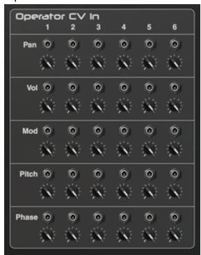
The Operator CV In group lets you control pan, volume, FM/RM modulation amount, pitch, and phase for the six operators.
