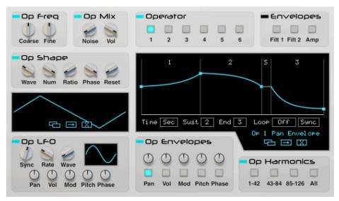
There are six operators, selectable from the Operator buttons. When an operator is selected its parameters are available in the Cyan labelled sections and on the main display.
