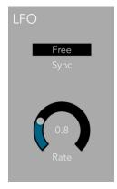
The LFO is a low frequency oscillator used for modulation. Its output is a triangle wave, a square wave, and sample and hold.
