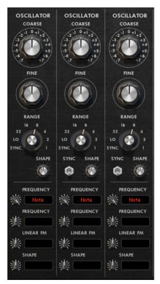
The upper left Oscillators section provides control over the three main oscillators. These oscillators have basic shapes, as well as a variable shape from VK-1.
