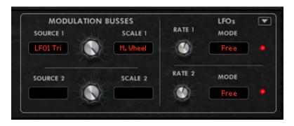
The two Mod Busses and two LFOs provide low frequency modulation signals for use in destinations throughout the synth.
