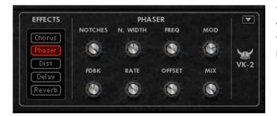
The phaser offers up to 6 notches, with configurable notch width and feedback, for a wide range of phasing sounds.
