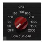
• Low Cut-off - CPS (Cycles Per Second) is the classic name for frequency before the standard name became Hertz. This selector switch controls the cutoff point of the high pass (low cut) filter in Hz.
