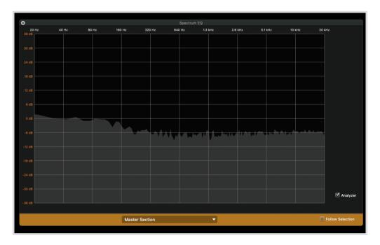
Attenuation at 30 Hz is shown below. Note that frequencies above the setting are also attenuated.
